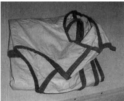
Figure 2. Folded RPE may be damaged in such a way as to cause sharp bends in the vinyl that deteriorate the lead-impregnated vinyl.
