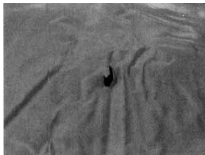
Figure 3. Routine RPE inspections help identify damage (e.g., tears, perforations, thinning, etc.) that compromise the effectiveness of this equipment.
